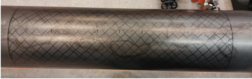
Figure 5.1: A traced toolpath on the mandrel at a low speed showing imperfections clearly.
