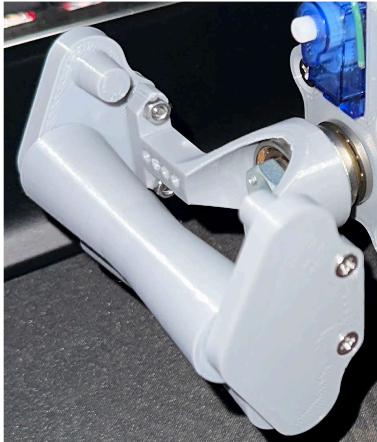
Figure 4.3: An early version of the wind eyelet showing how the sliding bearings work.
