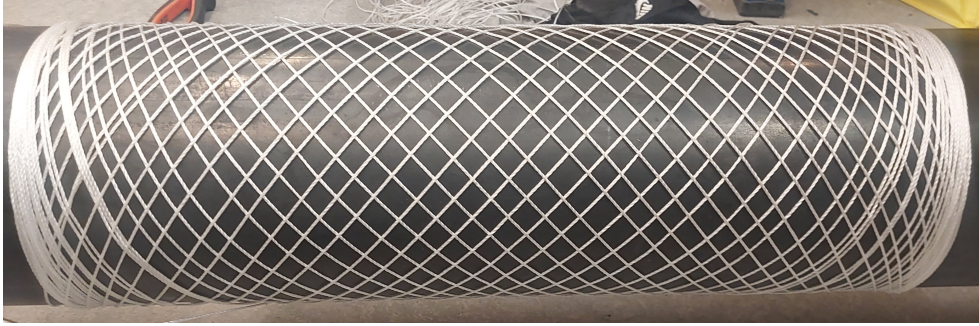
Figure 5.3: A relatively successful simulated filament lay-down example done at a medium speed with an unwashed mandrel.
